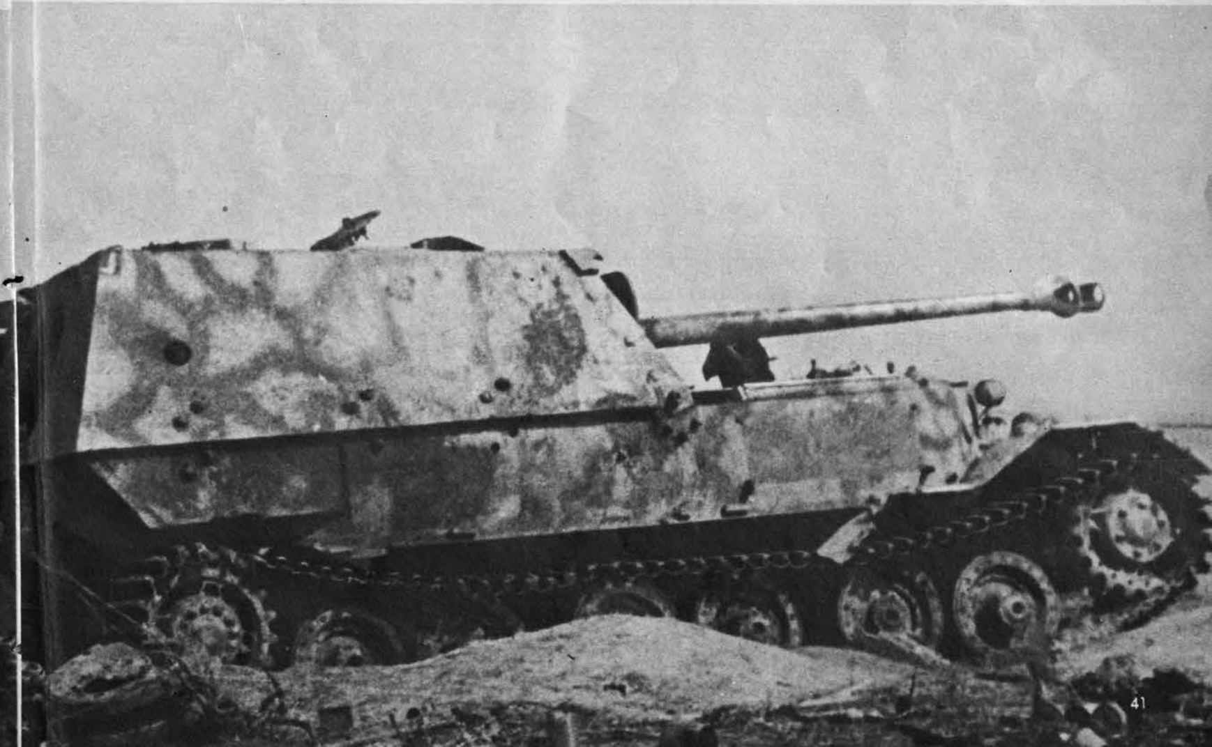
cause of the three distinct layers formed by the bow plate, hull and fighting compartment. Hull armor is eight in. thick in front, con-
